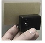
Handheld skimmers used by corrupt staff are very small, fitting in the palm of a hand.
